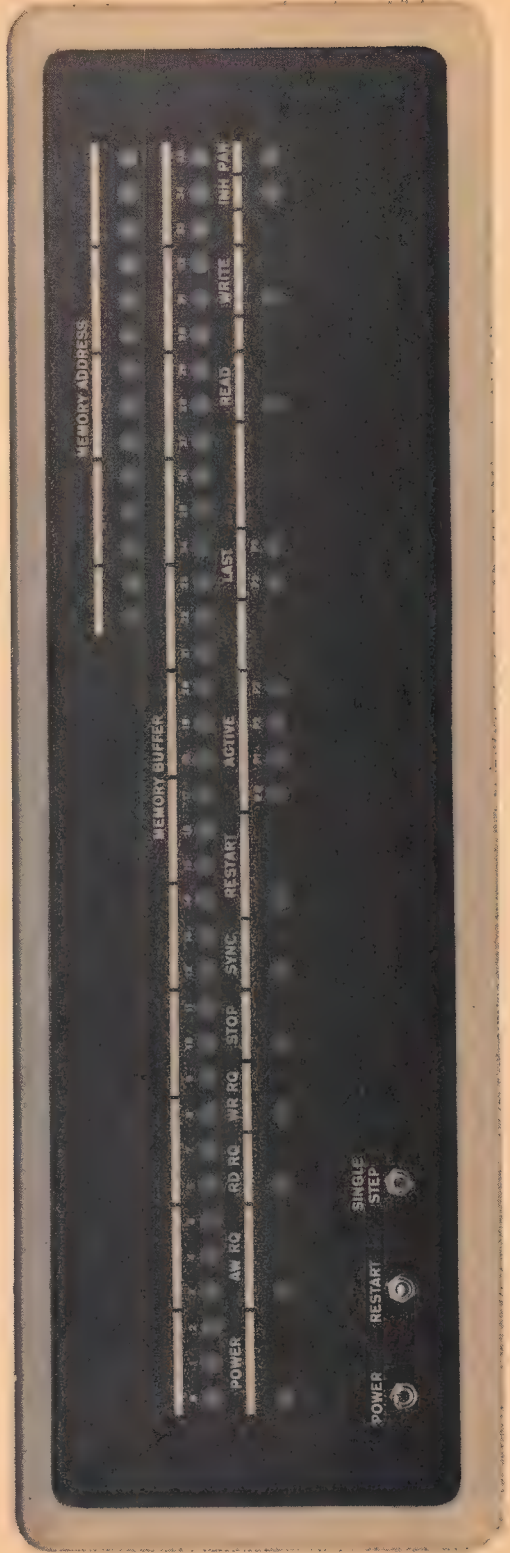
Indicator Panel, MB10 Core Memory (1.65 \mu s)
